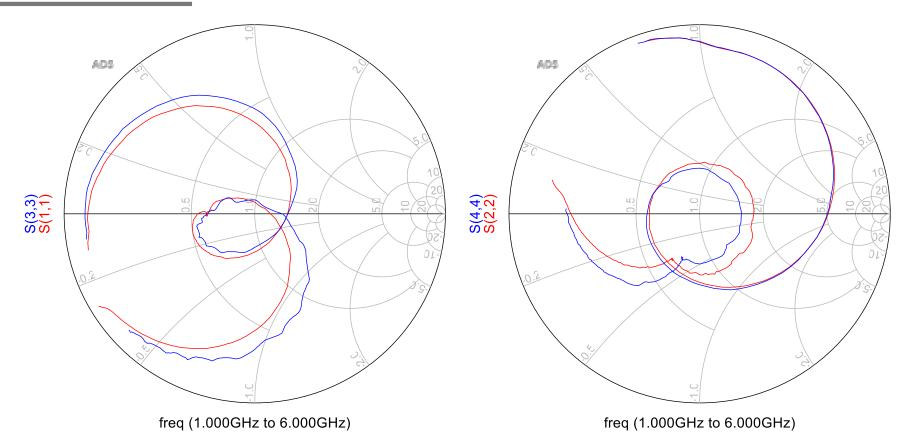
**Red curve – ADS simulation Blue curve – Measurement**
