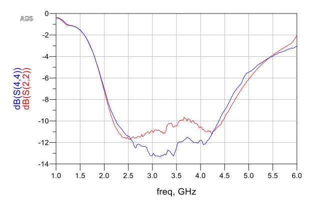
Red curve - ADS simulation **Blue curve – Measurement**
