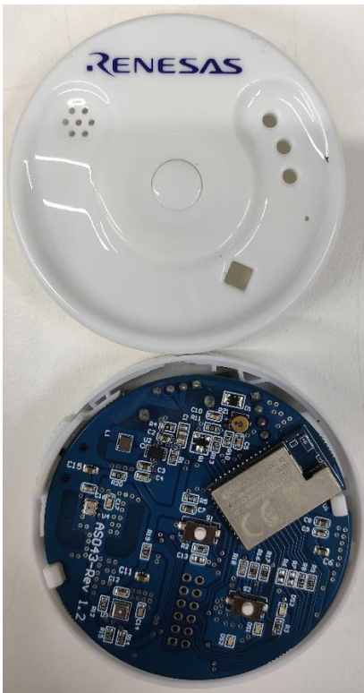
Figure 1. AS043 Flammable Gas Leakage Detector Board
