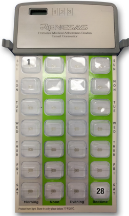
Figure 5: Smart Connector with Printed Foil Blister Pack
