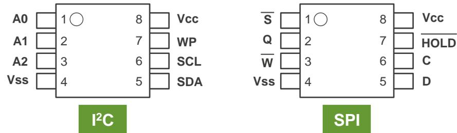
Pin Arrangement : 8-pin SOP / 8-pin TSSOP (Top View)
