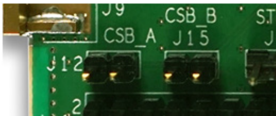
Figure 80. Jumpers for Serial Programming Connections
