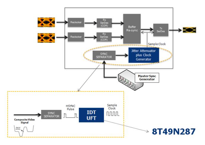
Figure 4: Example 8T49N287 Genlock Use Case
