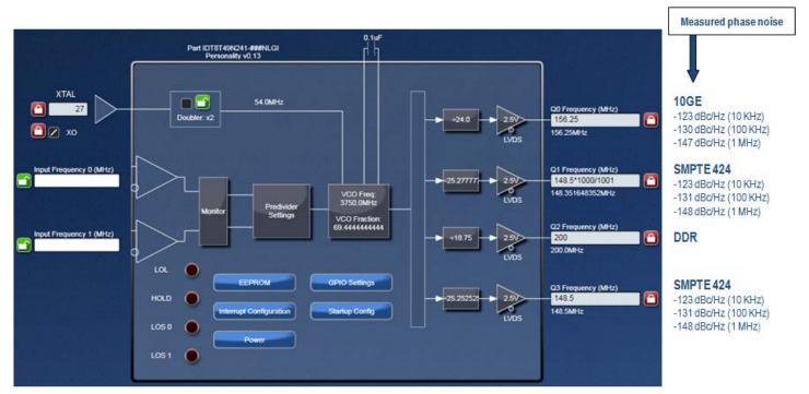
Figure 3a: Corresponding 8T49N241 Timing Commander GUI Configuration
