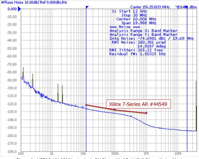
Figure 2: UFT3G 156.25MHz "typical" PN Plot, with AR #44549 Phase Noise Mask
