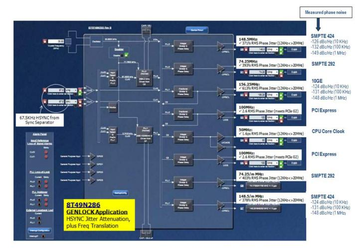
Figure 4b: Corresponding 8T49N287 Timing Commander GUI Configuration
