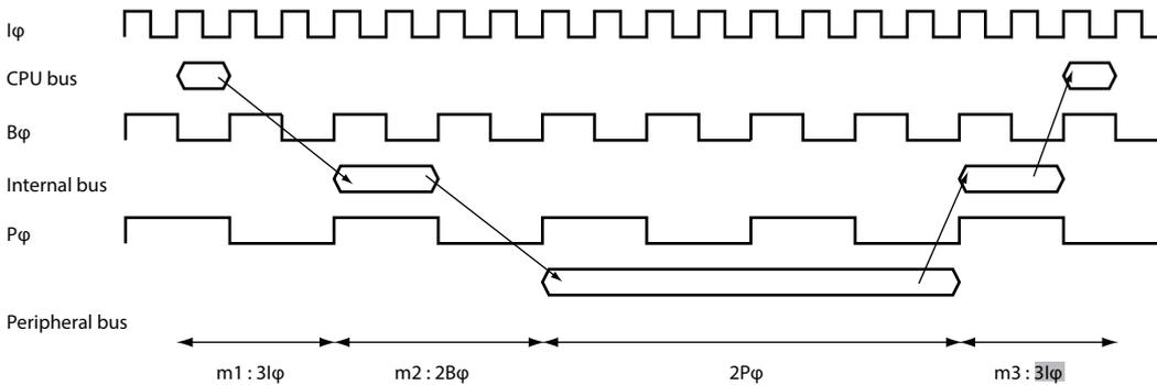
Figure 10.46 Timing of Read Access to On-Chip Peripheral I/O Registers and On-Chip RAM (for Data Retention) When  $I\phi:B\phi:P\phi = 4:2:1$
