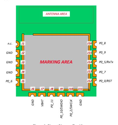
Figure 2: Pinout Diagram Top View
