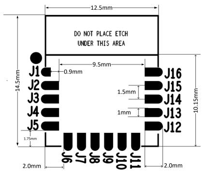
**Figure 4: Module Footprint Top View**
