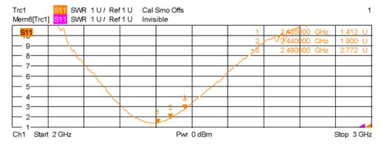
Figure 11: VSWR Installed in the Upper Left Corner (Position #1) of Evaluation Board
