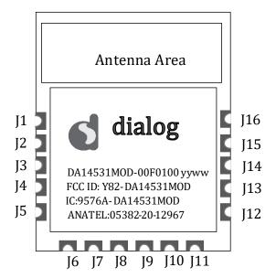
Figure 5: Module Shield Marking
