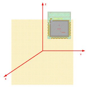
**Figure 14: Measurement Plane Definition**
