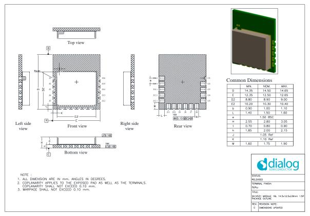
Figure 3: Mechanical Drawing
