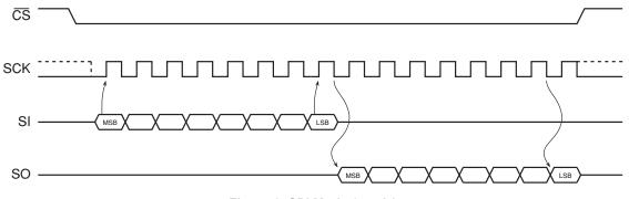
Figure 6. SPI Mode 0 and 3
