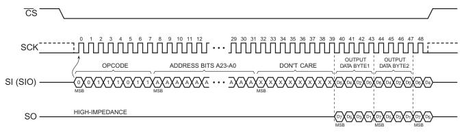
Figure 9. Dual-Output Read Array
