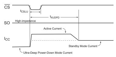
Figure 26. Exit Ultra-Deep Power-Down (Chip Select Toggle)
