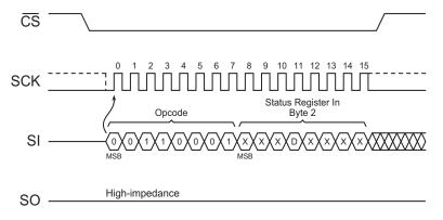
Figure 20. Write Status Register Byte 2
