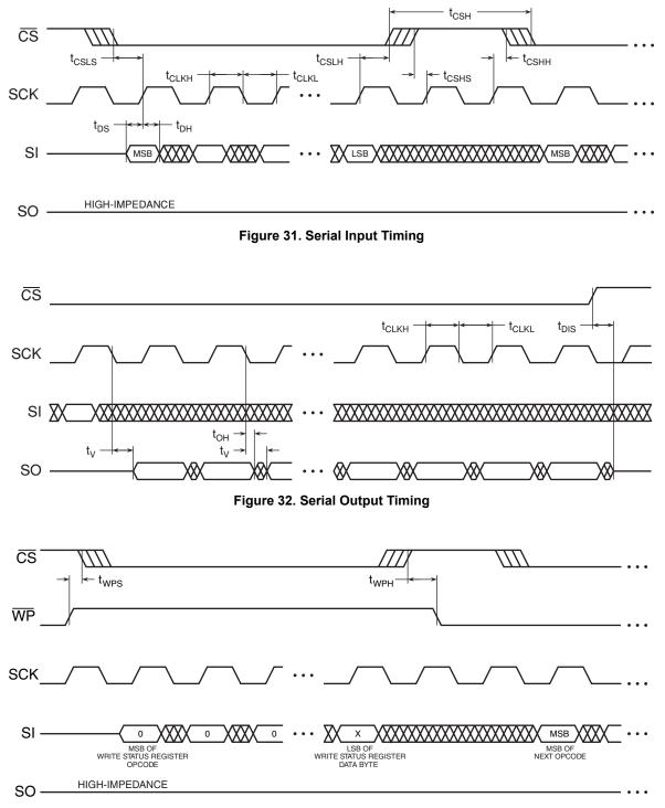
Figure 33. WP Timing for Write Status Register Command When BPL = 1
