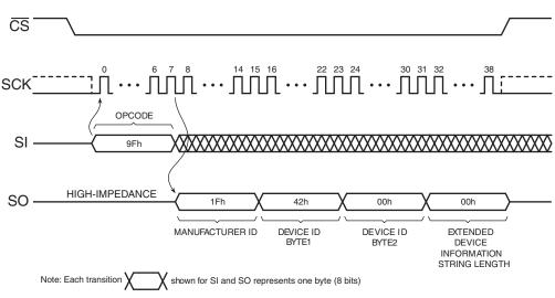
Figure 21. Read Manufacturer and Device ID
