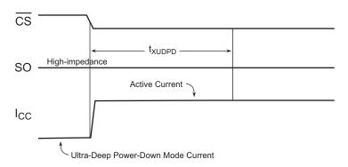
Figure 27. Exit Ultra-Deep Power-Down (Chip Select Low)
