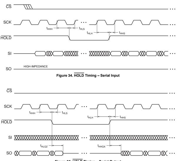
Figure 35. HOLD Timing – Serial Output
