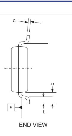
1. This drawing is for general information only. See JEDEC Drawing MO-153, Variation AA, for proper dimensions, tolerances, daturns, etc.
