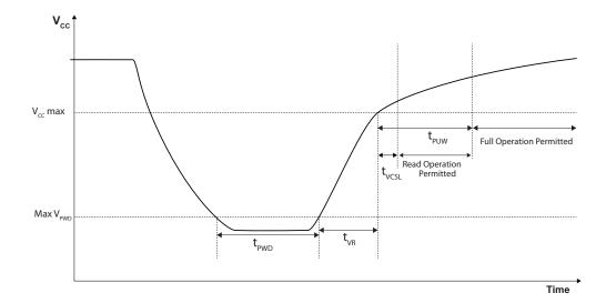
Figure 30. Power-Up Timing
