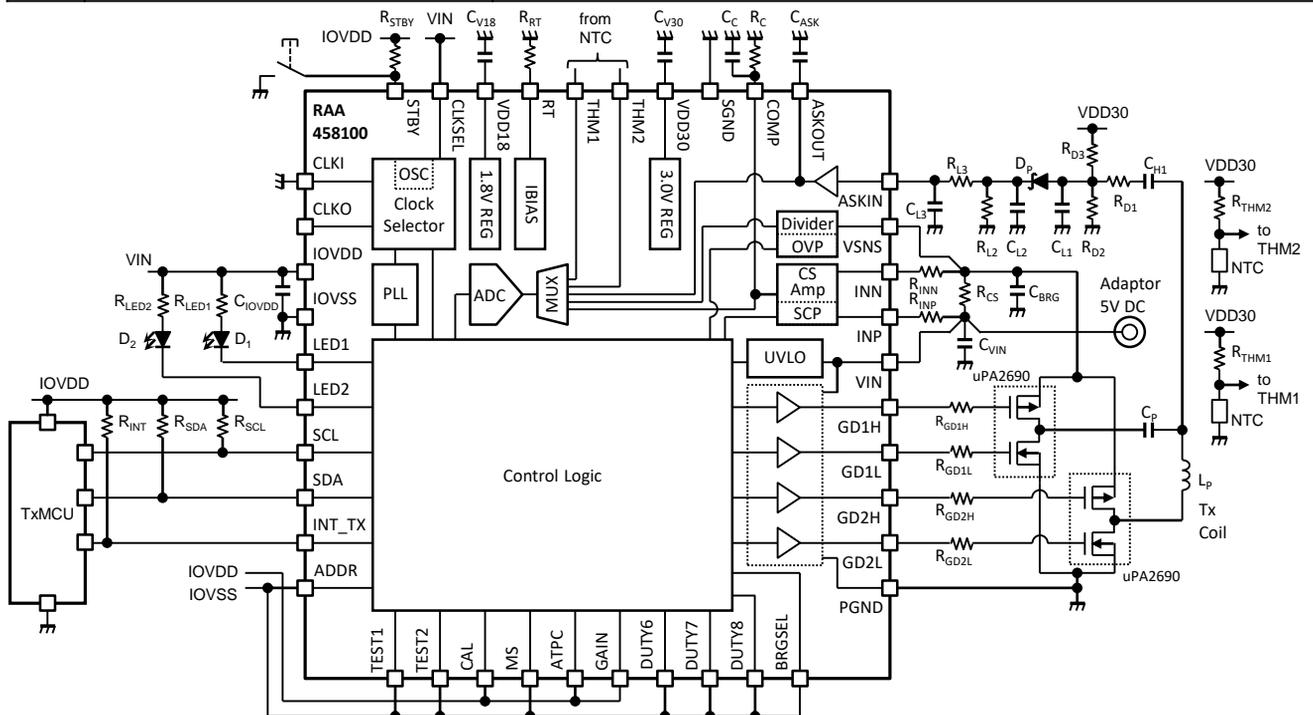
**Figure 2.1 Transmitter configuration for wireless charging system in AT2, AT3 and AT4**
