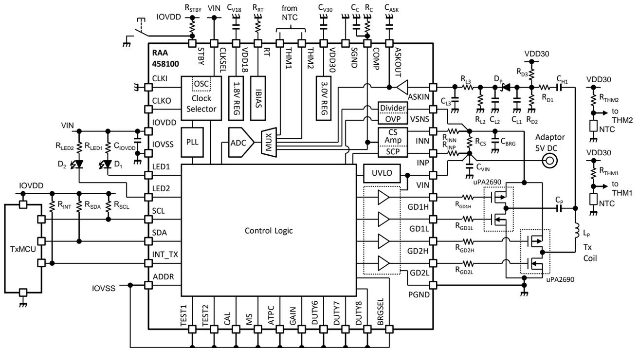
**Figure 2.2 Transmitter configuration for wireless charging system in MC1**
