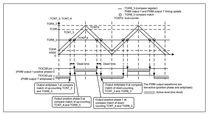
Figure 6 Complementary PWM Output Waveforms
