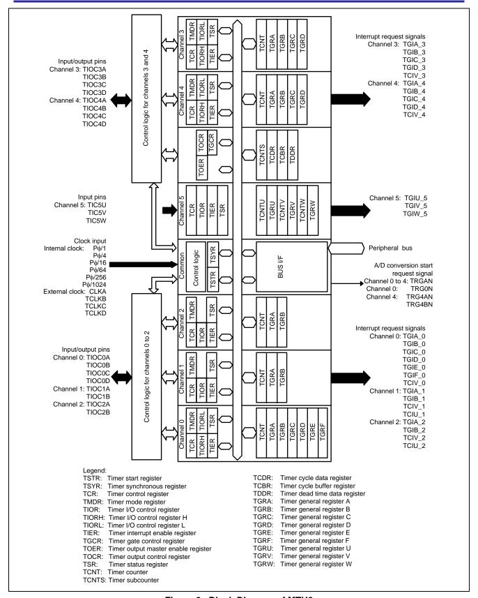
Figure 2 Block Diagram of MTU2
