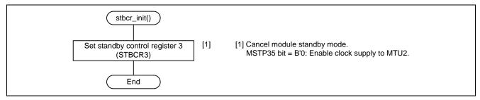
Figure 11 Initialization: Release from Standby
