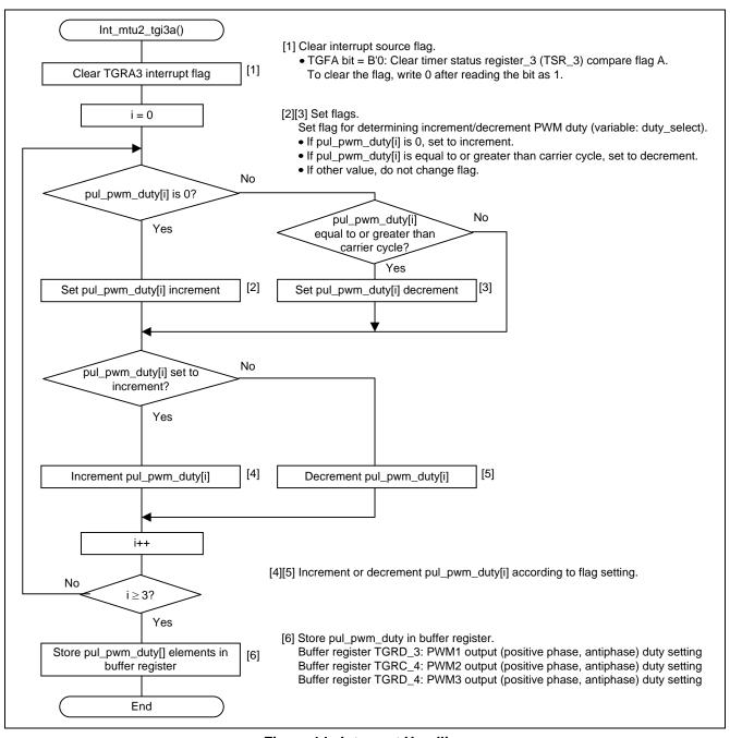
Figure 14 Interrupt Handling
