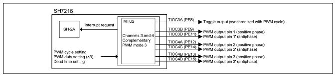
Figure 1 Three-Phase Complementary PWM Output (Complementary PWM Mode 3)
