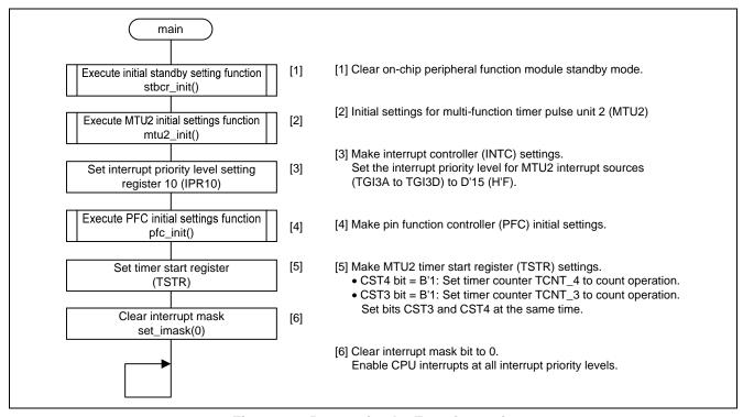
Figure 10 Processing by Function main
