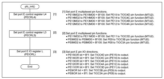
Figure 13 Initialization of Pin Function Controller (PFC)
