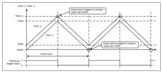
Figure 8 Operation for Toggling an Output in Synchronization with the PWM Cycle
