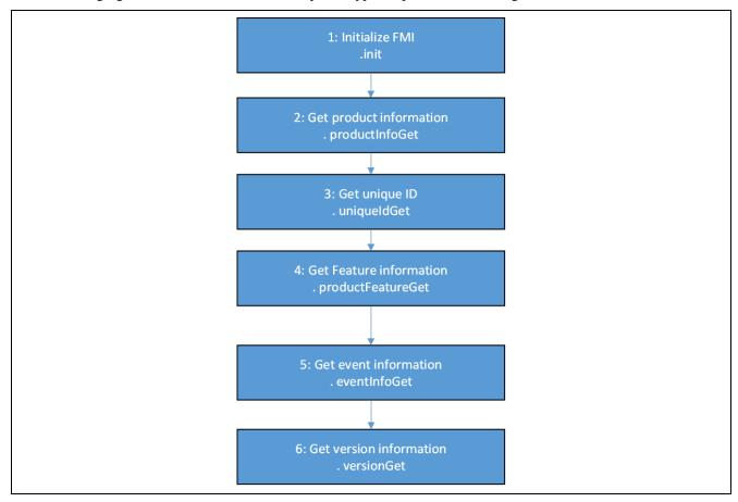
Figure 3 Flow Diagram of a Typical FMI HAL Module Application
