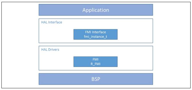
Figure 1 FMI HAL Module Block Diagram
