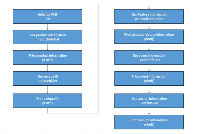
Figure 4 FMI HAL Module Application Project Flow Diagram
