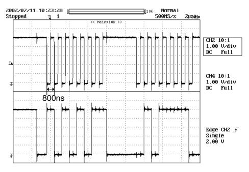
The result of data transmit with Clocked Serial communication.
