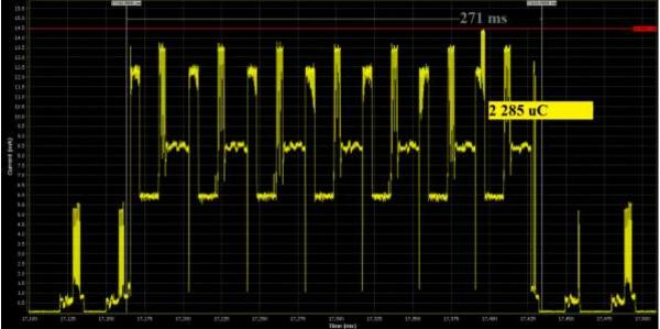
2. Every 12 packets (240 bytes) sent over the air, a WRITING operation is done. (time needed to receive 12 packets + writing operation: 92 ms, charge: 154 μC @3V).
