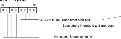
This setting reset Base Timers in Groups 0 to 3. Base Timer of Group i starts counting from 000016 by selecting a count source of Base Timer with register GiBCR0 and then set bit BTS = 1 in register GiBCR1.
