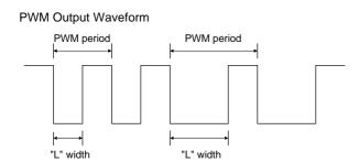
When Group 0 is selected, up to three PWM waveform having the same period can be output. In this case, the low-state of each waveform can be controlled by each channel.
