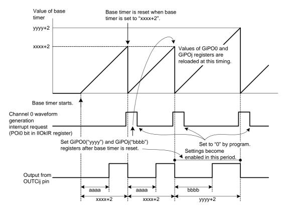
Note: "xxxx" is an initial value of the GiPO0 register and "aaaa" is of the GiPOj register.
