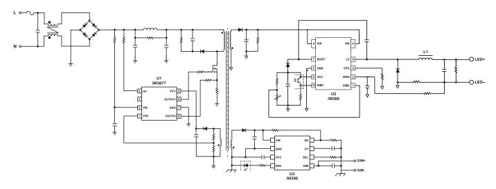
Figure 3.3 : iW388 Dimmable LED Driver Application with iW3677 Front-End Power Factor Correction Flyback and iW350 Interface IC
