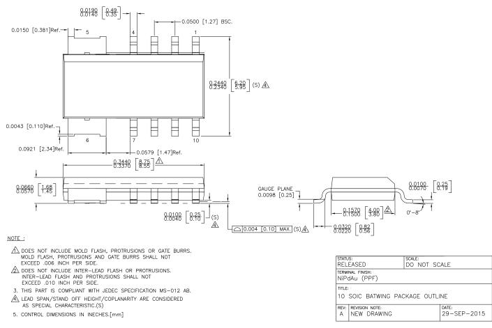
Figure 6.1 : 10-Lead SOIC Batwing Package Outline Drawing
