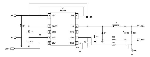
Figure 3.2 : iW388 Typical Application Circuit for CV/CC variants
