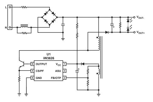
Figure 3.1 : iW3626 Typical Application Circuit (Non-isolated Application)
