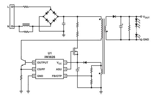
Figure 3.2 : iW3626 Typical Application Circuit (Isolated Application)
