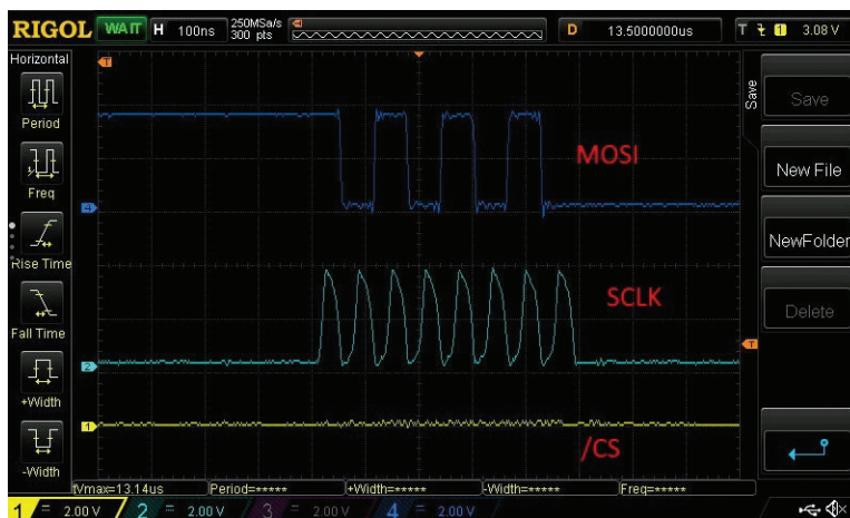
Figure 4: With no overshoot apparent, the serial flash memory's charge pump was able to operate correctly and provide reliable functionality
