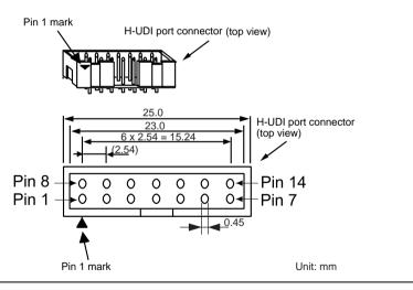
Figure 1.2 Pin Assignments of the H-UDI Port Connector (14 Pins)
