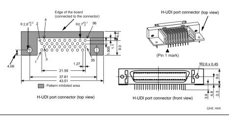
Figure 1.1 Pin Assignments of the H-UDI Port Connector (36 Pins)
