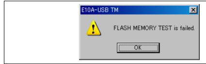
Figure 14 Error Message of the Flash Memory Test (Example)
