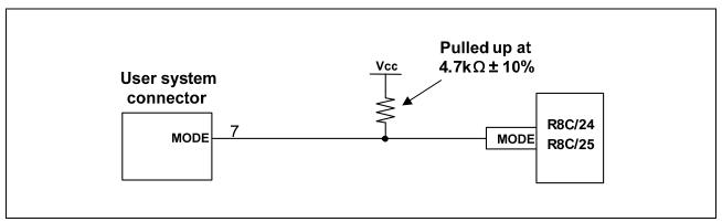
Figure 5.2 E8a Emulator and MODE Pin Connection
