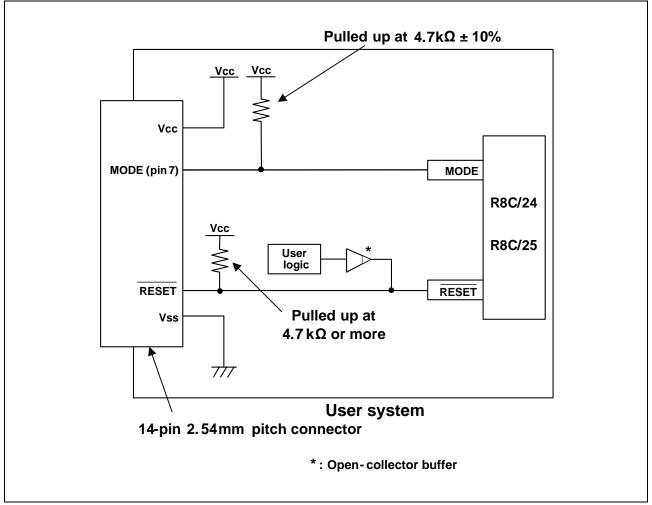
Figure 5.1 Example of an E8a Connection
