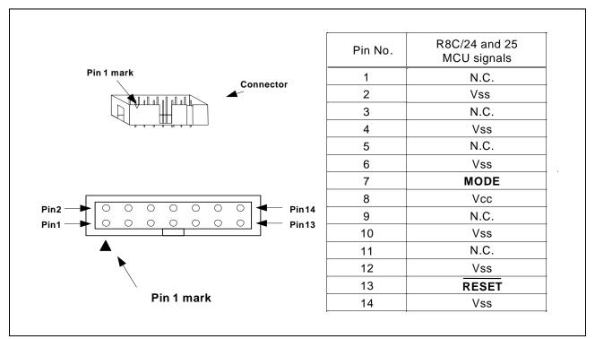
Figure 4.1 E8a Connecting Connector Pin Assignments
