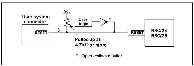
Figure 5.3 Example of a Reset Circuit
