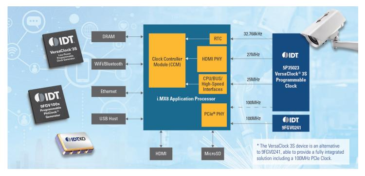
IDT's VersaClock<sup>®</sup> 3S family of programmable clock generators simplify system design by replacing multiple discrete timing components. This reduces both bill of materials (BOM) and board space, lowering system design costs. These devices offer a combination of low power consumption, flexibility and performance and are the perfect clocking solution to supply multiple external reference clocks to the NXP i.MX family of processors.
