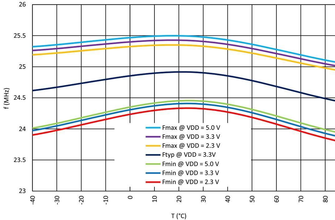
Figure 72: Oscillator1 Frequency vs. Temperature, OSC1 = 25 MHz
