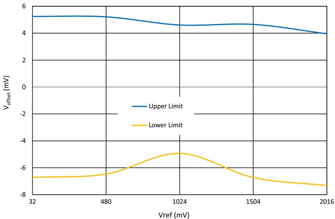
Figure 58: MS ACMP Input Offset Voltage vs. V<sub>ref</sub> at T = -40 °C to 85 °C
