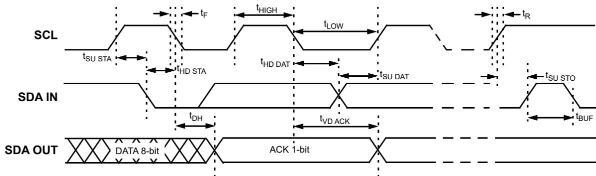
Figure 84: I<sup>2</sup>C General Timing Characteristics
