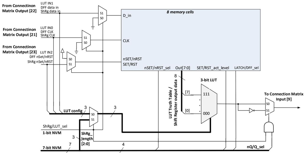
Figure 19: 3-bit LUT5 or DFF7 or Shift Register 1
