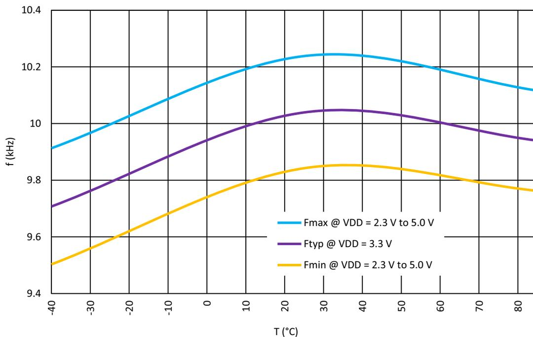
Figure 71: Oscillator0 Frequency vs. Temperature, OSC0 = 10 kHz
