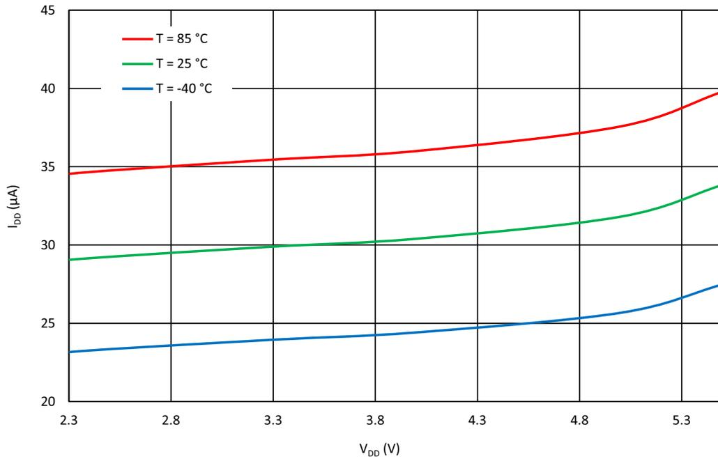
Figure 59: Current Consumption vs. V<sub>DD</sub> for Regular Mode, External Vref, V<sub>IN+</sub> = V<sub>DD</sub>, V<sub>IN-</sub> = GND
