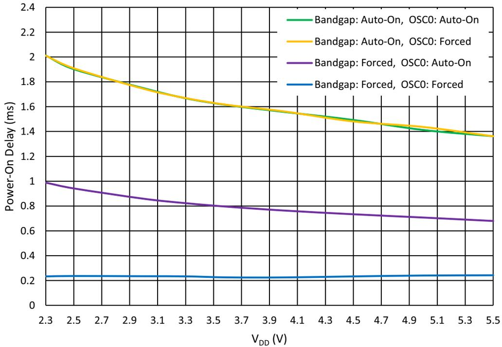
Figure 57: MS ACMP Power-On Delay vs. V<sub>DD</sub>, Sampling Mode, T = -40 °C to 85 °C
