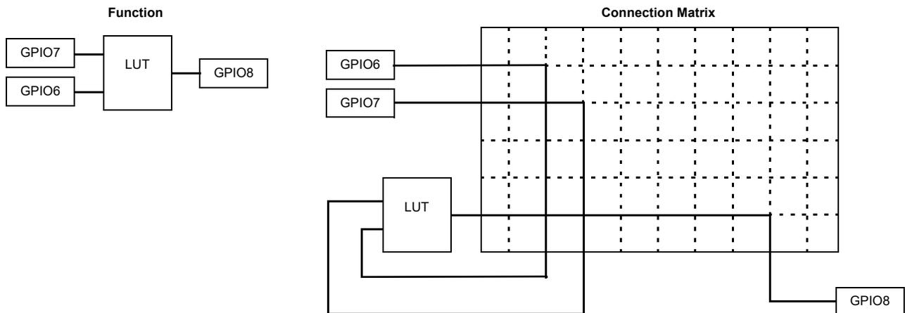
Figure 13: Connection Matrix Usage Example
