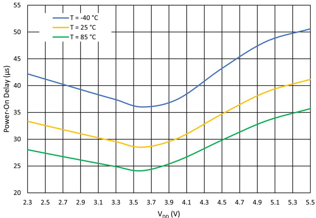
Figure 56: MS ACMP Power-On Delay vs. V<sub>DD</sub>, Regular Mode
