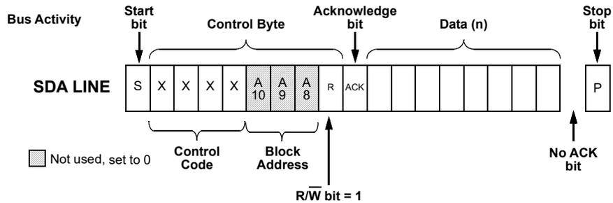
Figure 87: Current Address Read Command,  $\overline{R/W} = 1$
