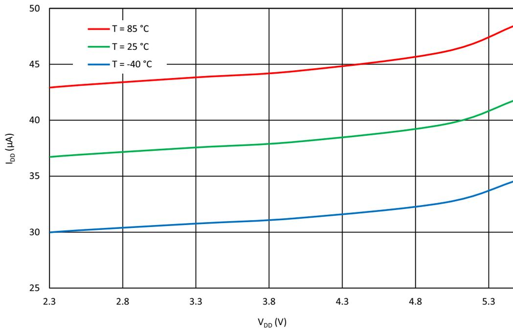
Figure 60: Current Consumption vs. V<sub>DD</sub> for Sampling Mode, 4 Channels, V<sub>IN+</sub> = 2048 mV, V<sub>IN-</sub> = 32 mV, Clock = 10 kHz
