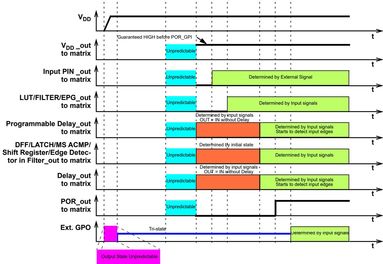
**Figure 81: Internal Macrocell States During POR Sequence**
