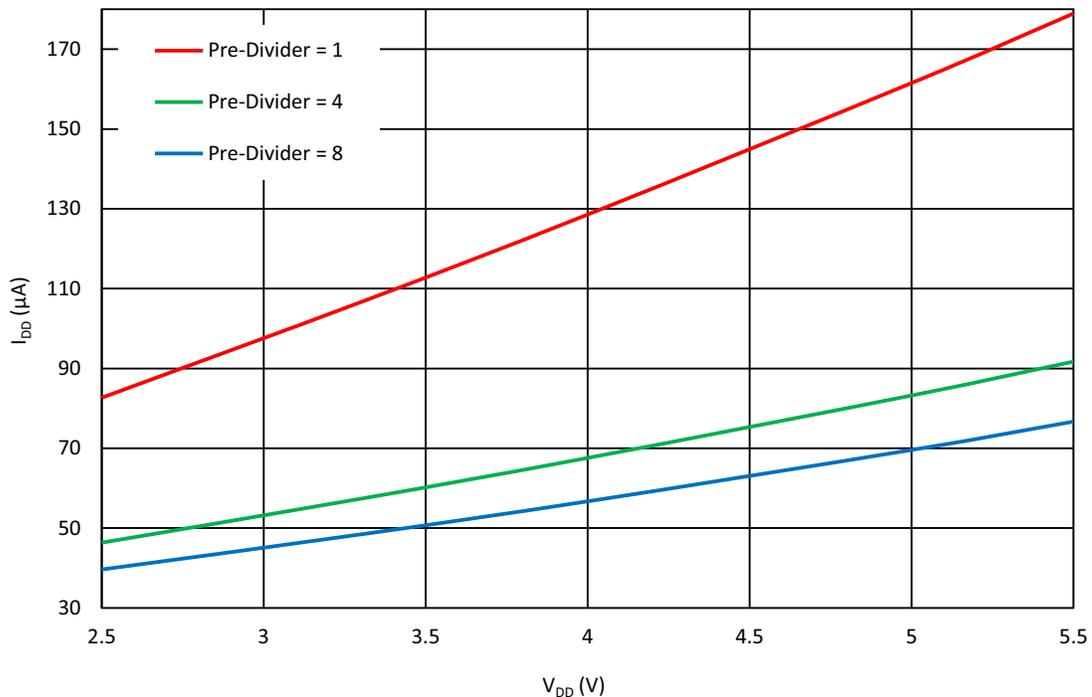
Figure 79: OSC1 Current Consumption vs. V<sub>DD</sub>, T = -40 °C to 85 °C, OSC1 = 25 MHz
