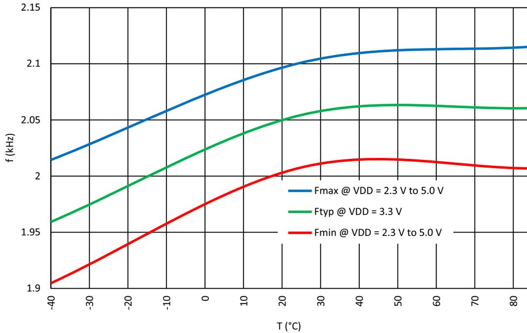
Figure 70: Oscillator0 Frequency vs. Temperature, OSC0 = 2.048 kHz
