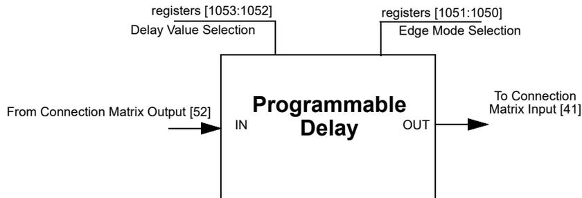
Figure 61: Programmable Delay
