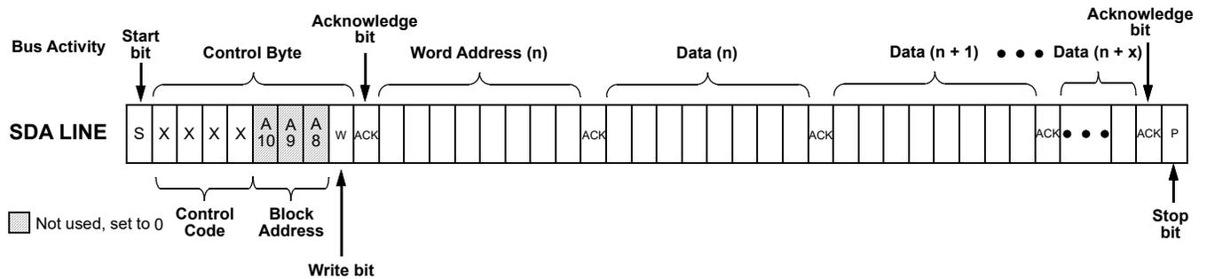
Figure 86: Sequential Write Command
