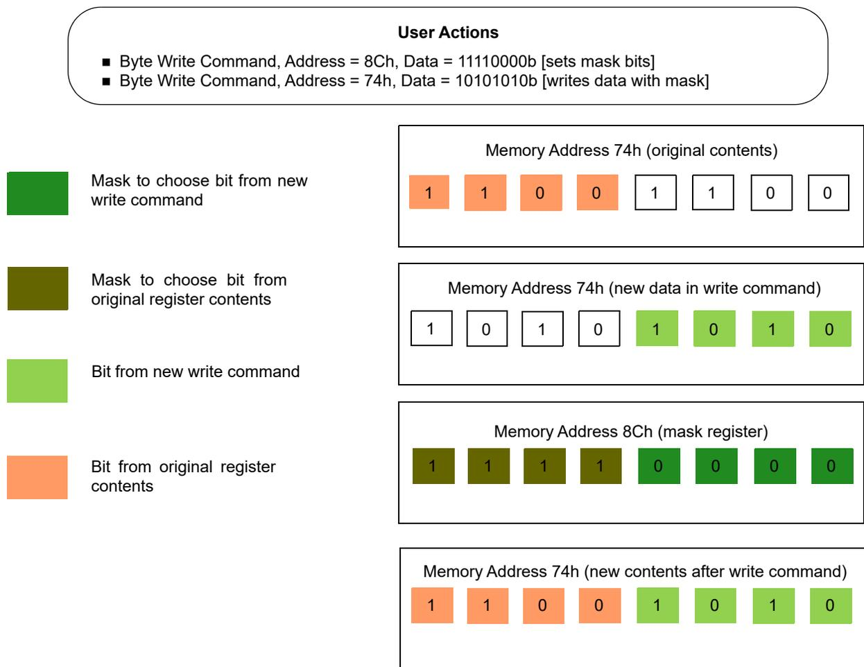
Figure 91: Example of I<sup>2</sup>C Byte Write Bit Masking
