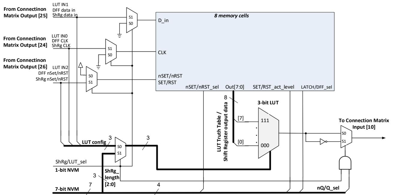
Figure 20: 3-bit LUT6 or DFF8 or Shift Register 2
