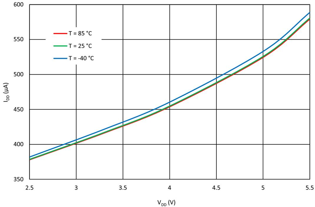
Figure 78: OSC0 Current Consumption vs. V<sub>DD</sub> (All Pre-Dividers), OSC0 = 10 kHz
