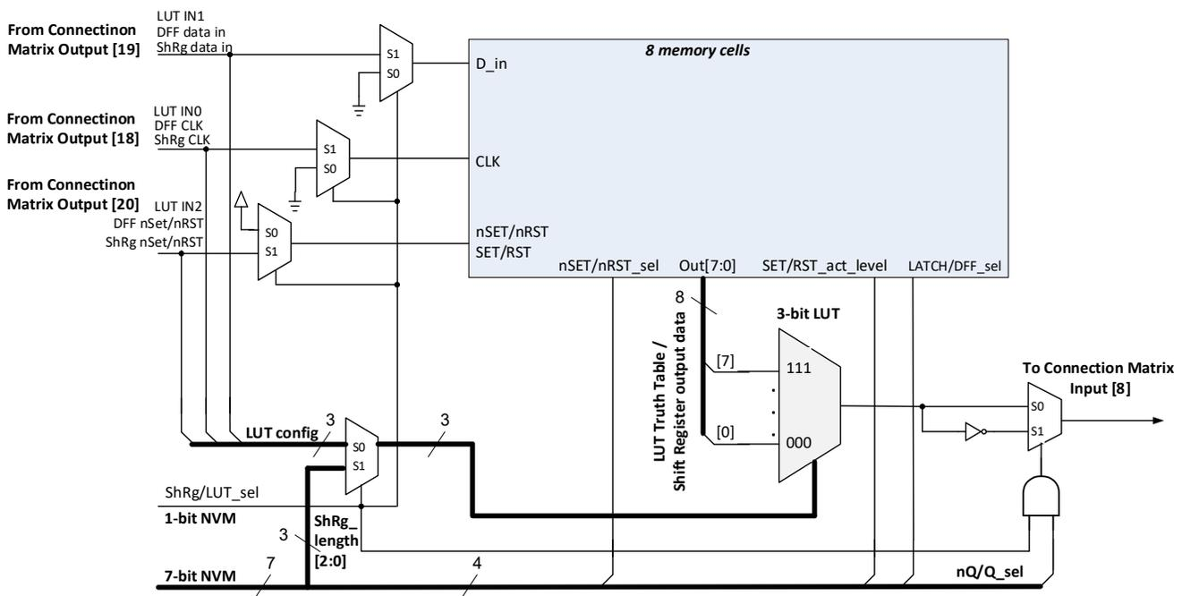
Figure 18: 3-bit LUT4 or DFF6 or Shift Register 0
