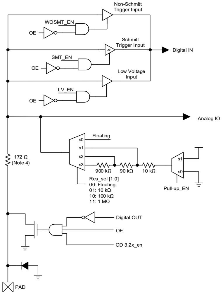
Figure 4: GPIO with I<sup>2</sup>C Mode IO Structure Diagram
