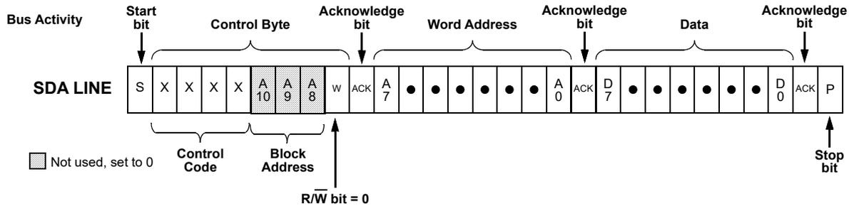
Figure 85: Byte Write Command,  $\overline{R/W} = 0$
