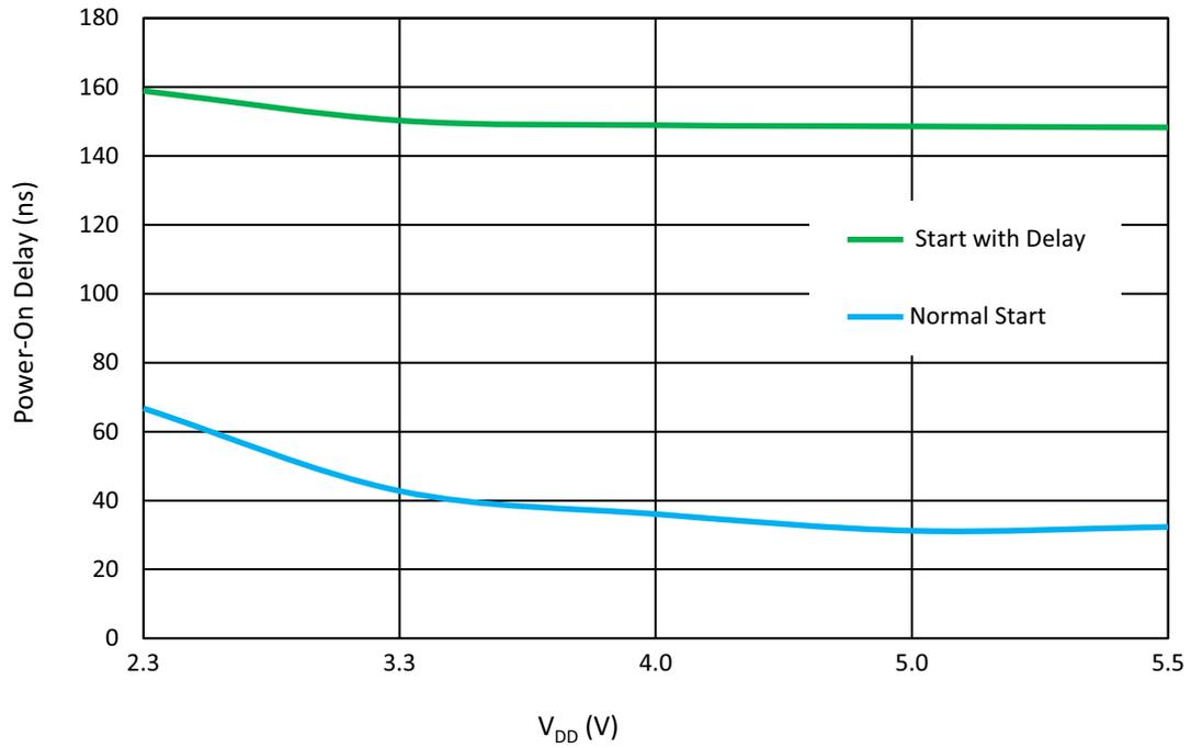
Figure 69: Oscillator1 Maximum Power-On Delay vs. V<sub>DD</sub> at T = 25 °C, OSC1 = 25 MHz
