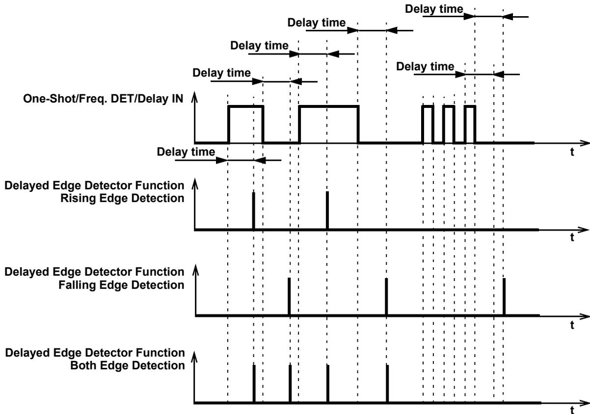
Figure 48: Delayed Edge Detection Mode Timing Diagram
