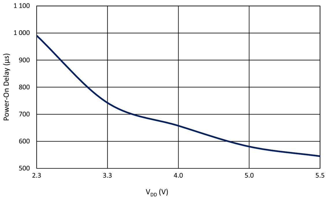
Figure 68: Oscillator0 Maximum Power-On Delay vs. V<sub>DD</sub> at T = 25 °C, OSC0 = 2.048 kHz/10 kHz
