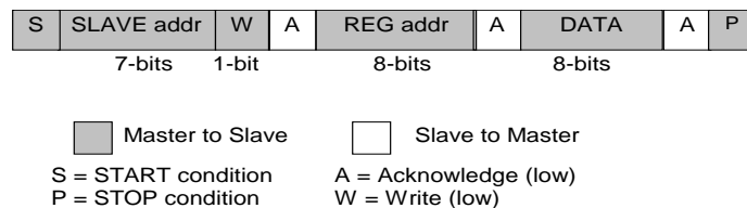
Figure 24: I 2 C Byte Write (SDA line)
