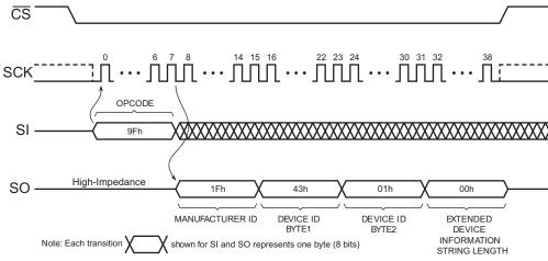
Figure 30. Read Manufacturer and Device ID
