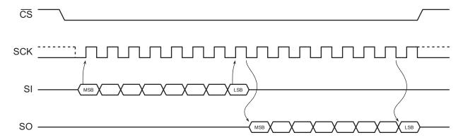
Figure 7. SPI Mode 0 and 3
