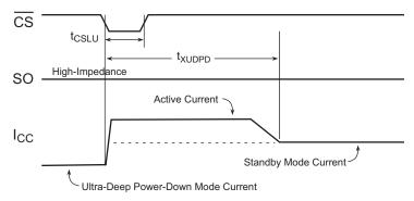
Figure 34. Exit Ultra-Deep Power-Down (Chip Select Toggle)
