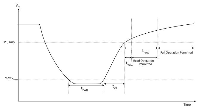
Figure 37. Power-Up Timing
