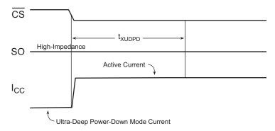
Figure 35. Exit Ultra-Deep Power-Down (Chip Select Low)
