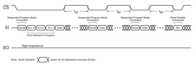
Figure 16. Sequential Program Mode – Waiting Maximum Byte Program Time
