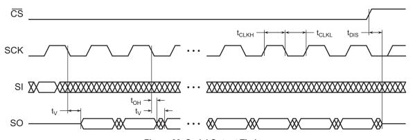
Figure 39. Serial Output Timing
