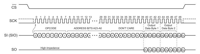
Figure 10. Dual-Output Read Array
