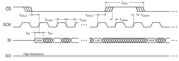
Figure 38. Serial Input Timing
