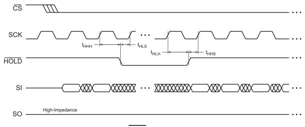
Figure 41. HOLD Timing – Serial Input
