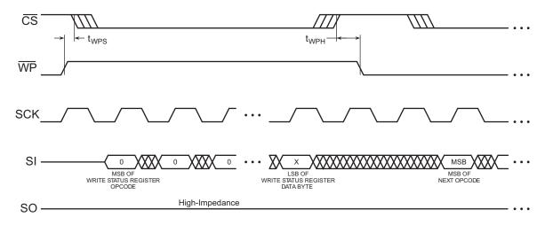
Figure 40. WP Timing for Write Status Register Command When BPL = 1
