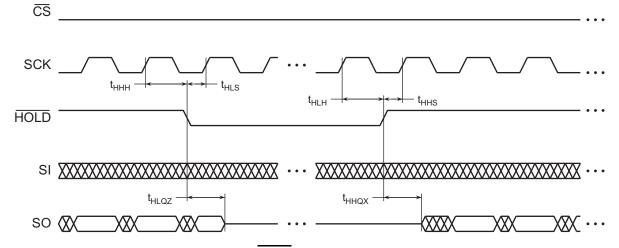
Figure 42. HOLD Timing – Serial Output
