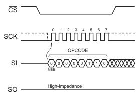
Figure 19. Write Enable
