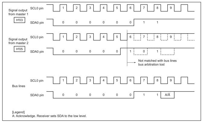
Figure 6 Loss of Bus Arbitration During Data Transmission
