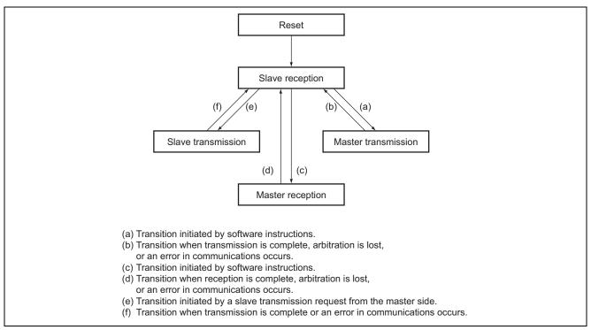
Figure 7 State Transition Diagram
