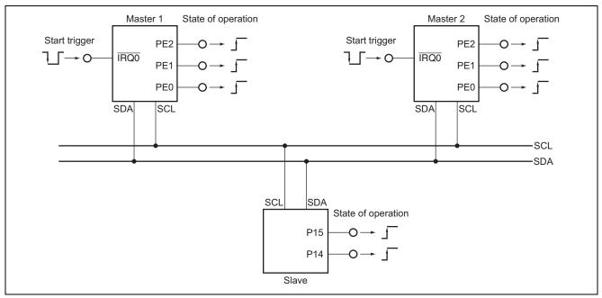
Figure 1 Connections for I<sup>2</sup>C Bus Interface Multi-Master Mode Communication
