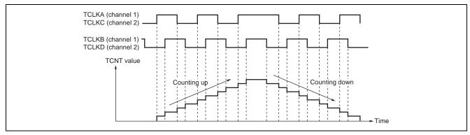
Figure 3 Example of Operation in Phase Counting Mode 1 (Channels 1 and 2)
