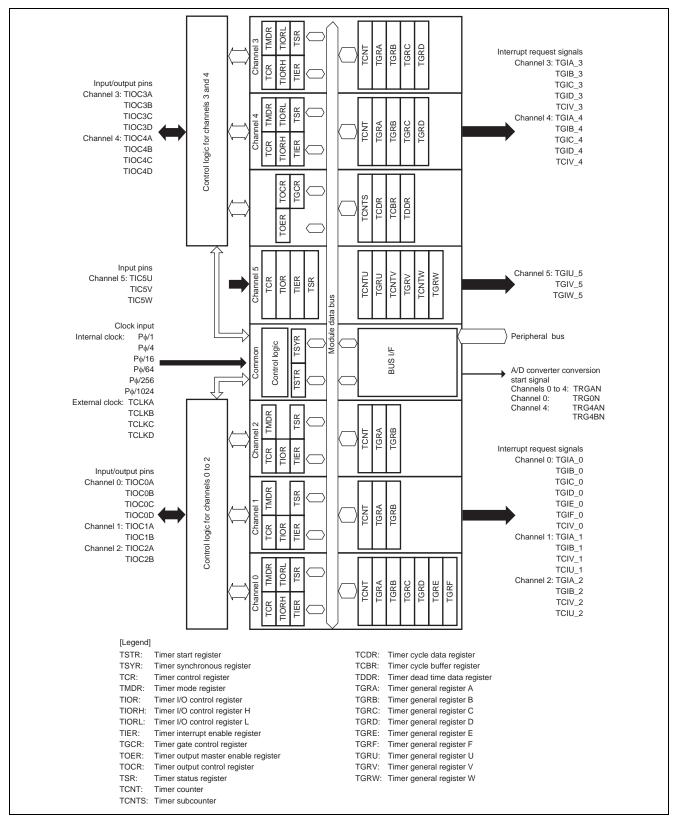
Figure 2 Block Diagram of MTU2
