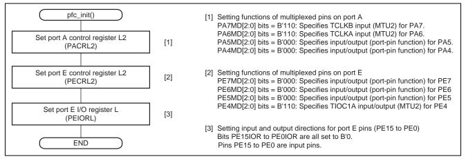
Figure 9 Flow for Setting PFC
