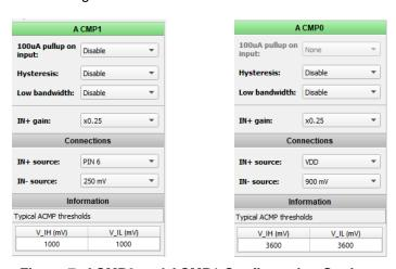
Figure 7: ACMP0 and ACMP1 Configuration Settings
