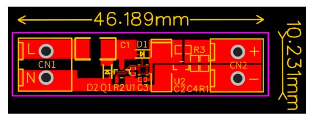
Figure 4: CCSS Regulator PCB Layout
