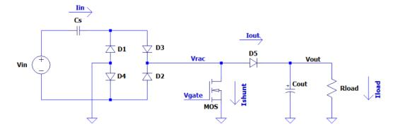
Figure 1: Capacitor-Coupled Switched Shunt Regulator
