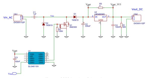
Figure 3: CCSS Regulator Schematic
