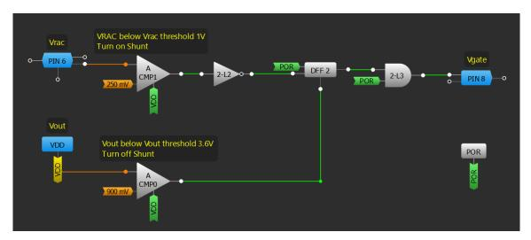
Figure 6: SLG46110 GreenPAK Design
