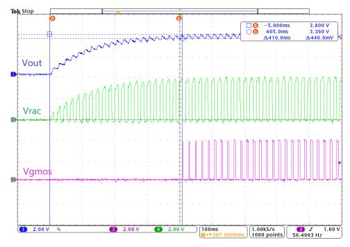
Figure 8: Waveforms of CCSS
