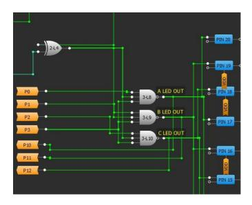
Figure 4. LED output circuit design
