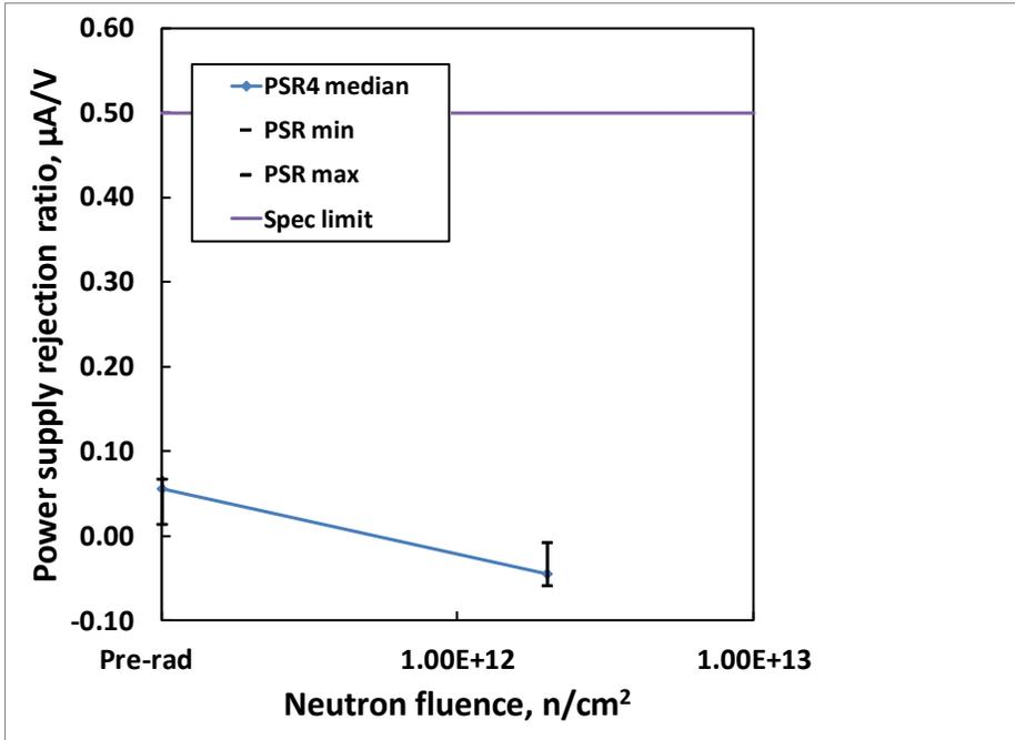
**Fig. 2:** ISL71590SEH power supply rejection ratio at 4.0V as a function of neutron irradiation, showing the median, minimum and maximum of the populations at each level. The sample size was 5 and the neutron fluence was  $2 \times 10^{12}$  n/cm<sup>2</sup>, with three control units. The post-total dose irradiation SMD limit is 0.50 µA/V maximum.
