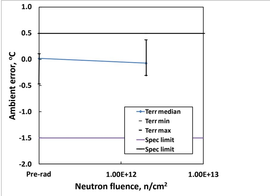
**Fig. 1:** ISL71590SEH temperature error as a function of neutron irradiation, showing the median, minimum and maximum of the populations at each level. The sample size was 5 and the neutron fluence was  $2 \times 10^{12}$  n/cm<sup>2</sup>, with three control units. The post-total dose irradiation SMD limits are -1.5°C to +0.5°C.
