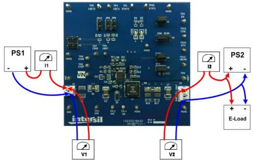
FIGURE 1. QUICK SETUP DIAGRAM
