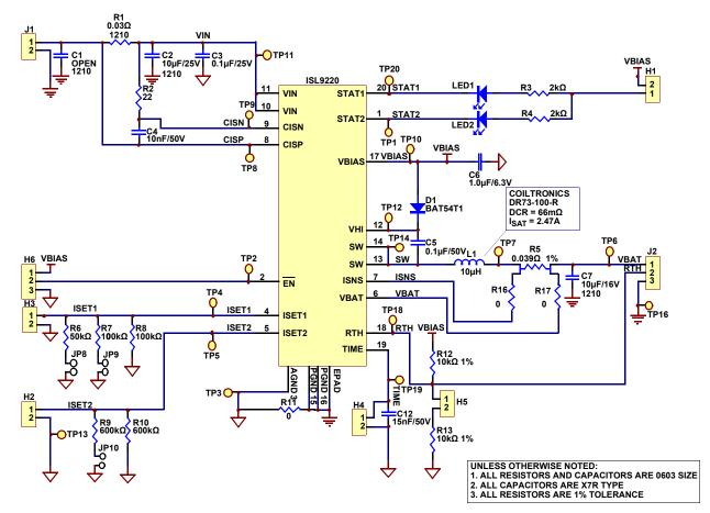
FIGURE 2. ISL9220, ISL9220A EVALUATION BOARD SCHEMATIC
