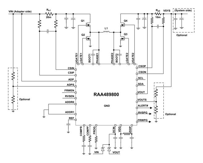
Figure 1. Typical Application Circuit in 4-Switch Buck-Boost Configuration
