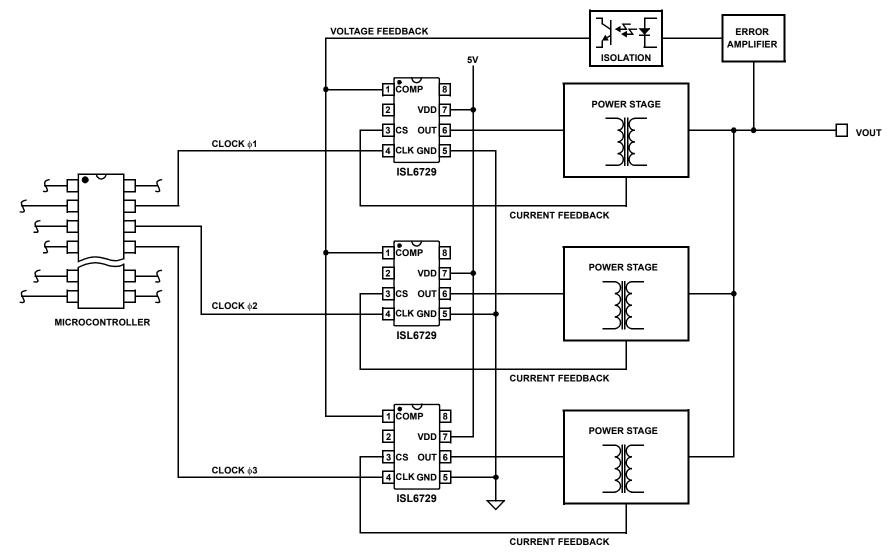
FIGURE 2. TYPICAL APPLICATION - INTERLEAVED MULTIPHASE ISOLATED CONVERTER
