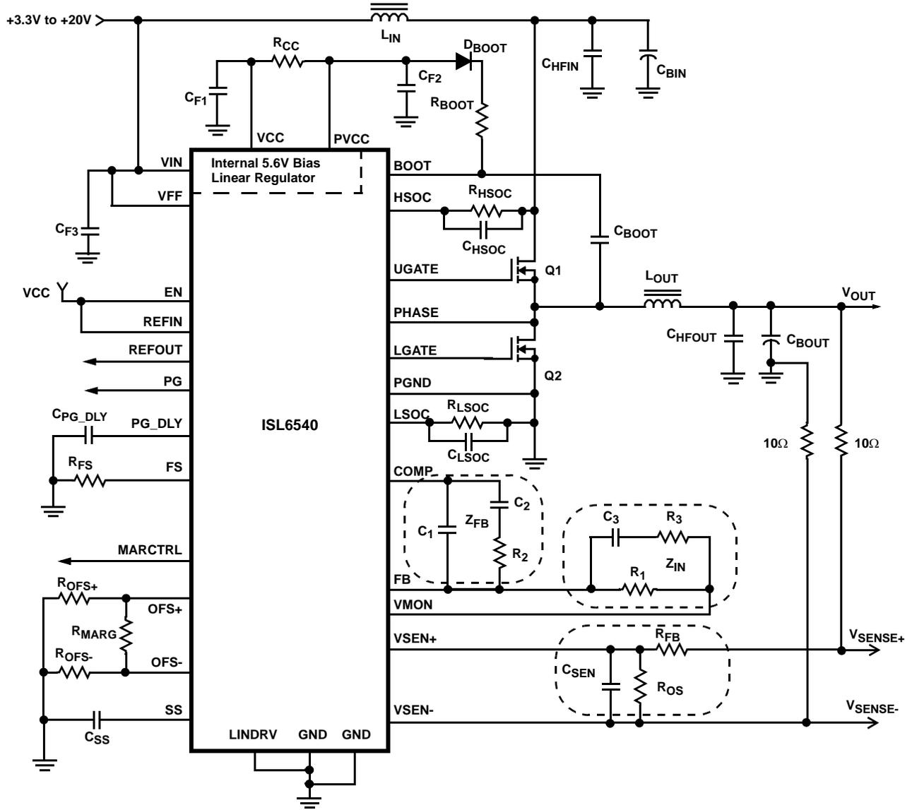
Typical Application II (External Linear Regulator without Remote Sense)
