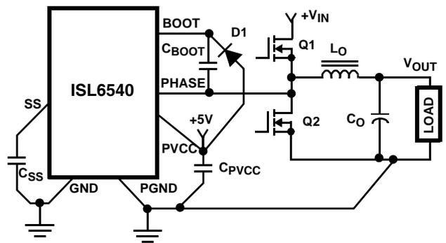
FIGURE 8. PRINTED CIRCUIT BOARD SMALL SIGNAL LAYOUT GUIDELINES
