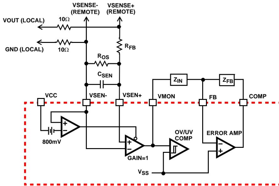
FIGURE 6. SIMPLIFIED UNITY GAIN DIFFERENTIAL SENSING IMPLEMENTATION
