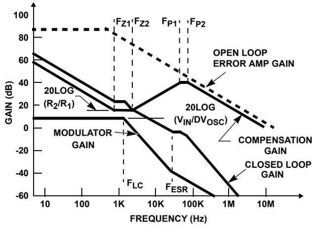
FIGURE 6. ASYMPTOTIC BODE PLOT OF CONVERTER GAIN
