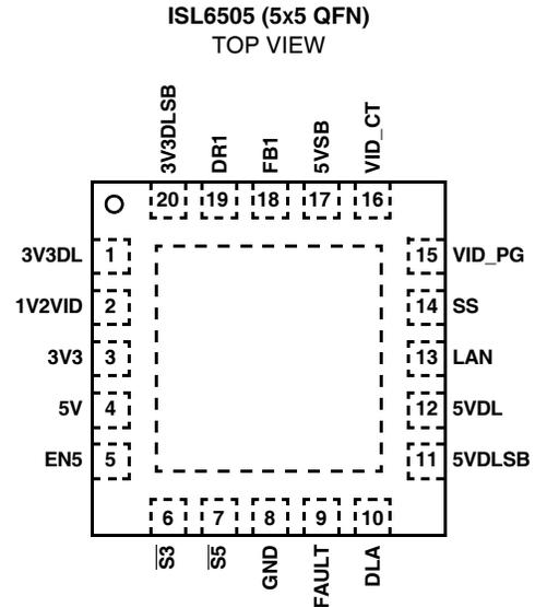
NOTE: The QFN bottom pad is electrically connected to the IC substrate, at GND potential. It can be left unconnected, or connected to GND; do NOT connect to another potential.
