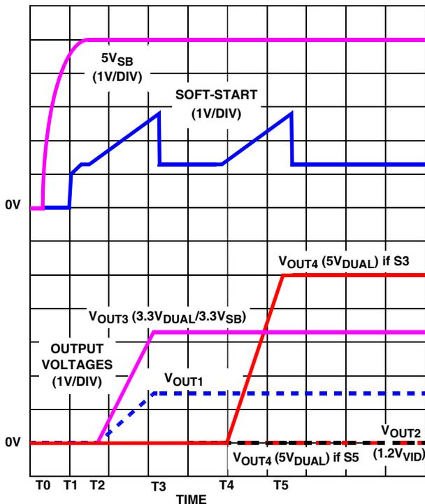
FIGURE 7. SOFT-START INTERVAL IN A SLEEP STATE;
