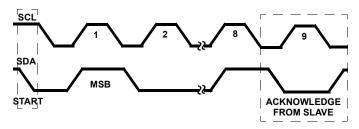
FIGURE 6. ACKNOWLEDGE ON THE I<sup>2</sup>C BUS
