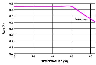
FIGURE 3. OUTPUT CURRENT DERATING (6x6 QFN)
