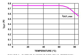
FIGURE 2. OUTPUT CURRENT DERATING (EPTSSOP)
