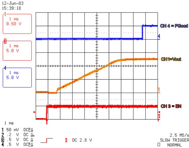
FIGURE 1. SOFT-START WAVEFORM
