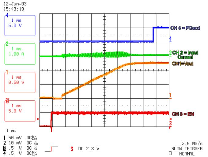
FIGURE 2. INRUSH CURRENT AT VIN 19V @ 52A
