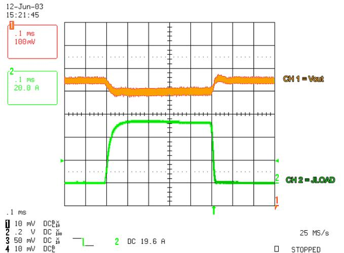
FIGURE 4. TRANSIENT WAVEFORM FROM 0A TO 52A
