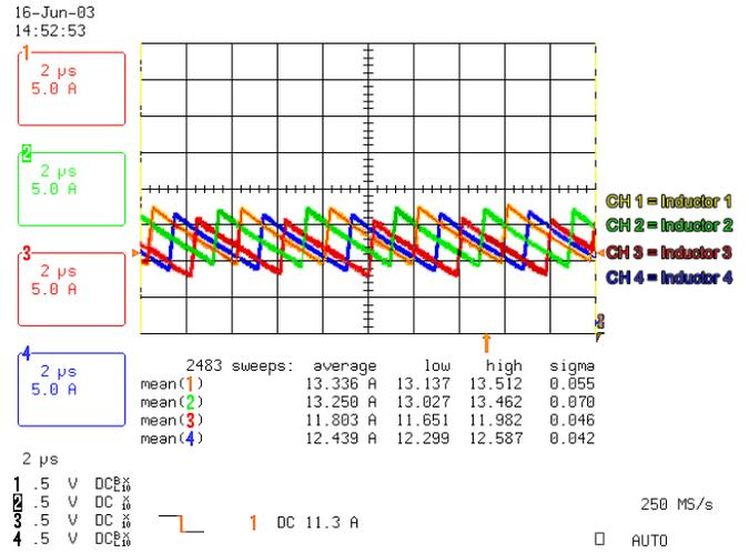
FIGURE 8. FOUR PHASE CURRENT BALANCE @ 52A
