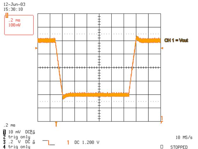
FIGURE 6. VID CHANGES FROM 1.60V TO 1.20V
