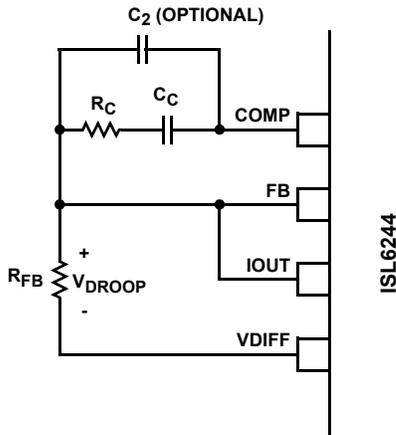
FIGURE 25. COMPENSATION CONFIGURATION FOR LOAD-LINE REGULATED ISL6244 CIRCUIT
