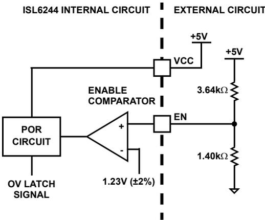
FIGURE 20. POWER SEQUENCING USING THRESHOLD-SENSITIVE ENABLE (EN) FUNCTION
