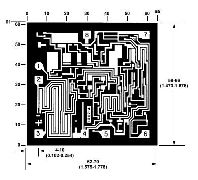
Dimensions in parenthesis are in millimeters and are derived from the basic inch dimensions as indicated. Grid graduations are in mils ( $10^{-3}$  inch).
