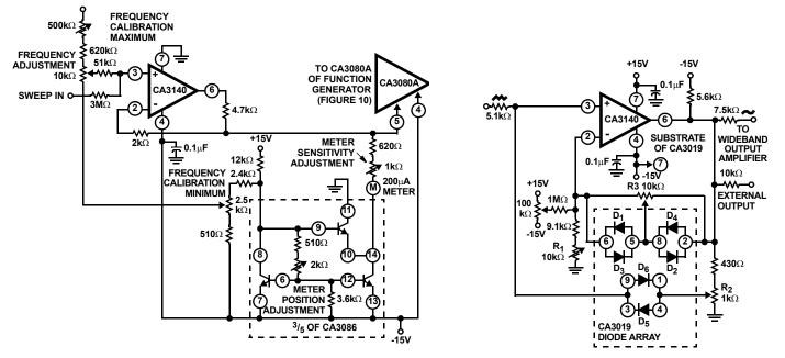
FIGURE 11. METER DRIVER AND BUFFER AMPLIFIER
