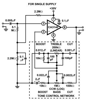
Bass treble boost and cut are  $\pm 15$ dB at 100Hz and 10kHz, respectively. Full peak-to-peak output is available up to at least 20kHz due to the high slew rate of the CA3140. The amplifier gain is 3dB down from its "flat" position at 70kHz.
