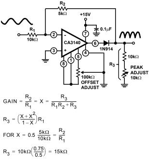
20V<sub>P-P</sub> Input BW (-3dB) = 290kHz, DC Output (Avg) = 3.2V
