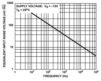
FIGURE 35. EQUIVALENT INPUT NOISE VOLTAGE vs FREQUENCY
