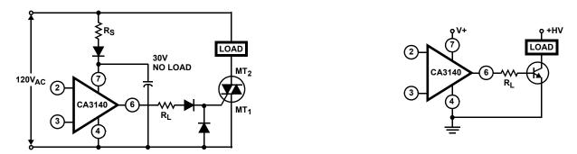
FIGURE 4. METHODS OF UTILIZING THE VCE(SAT) SINKING CURRENT CAPABILITY OF THE CA3140 SERIES
