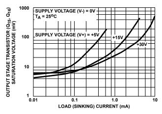
FIGURE 2. VOLTAGE ACROSS OUTPUT TRANSISTORS (Q<sub>15</sub> AND Q<sub>16</sub>) vs LOAD CURRENT
