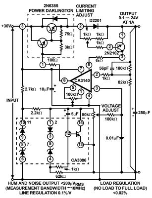
FIGURE 16. REGULATED POWER SUPPLY
