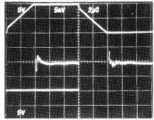
Top Trace: Output Signal; 5V/Div, 2μs/Div. Center Trace: Difference of Input and Output Signals through Tektronix Amplifier 7A13; 5mV/Div., 2μs/Div.
