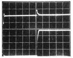
Top Trace: Output Voltage; 200mV/Div., 5µs/Div. Bottom Trace: Collector of load switching transistor, load = 1A; 5V/Div., 5µs/Div.
