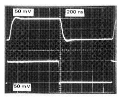
Top Trace: Output; 50mV/Div., 200ns/Div. Bottom Trace: Input; 50mV/Div., 200ns/Div. FIGURE 28B. SMALL SIGNAL RESPONSE
