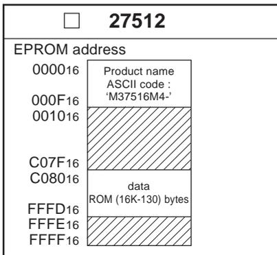
In the address space of the microcomputer, the internal ROM area is from address C080<sub>16</sub> to FFFD<sub>16</sub>. The reset vector is stored in addresses FFFC<sub>16</sub> and FFFD<sub>16</sub>.
