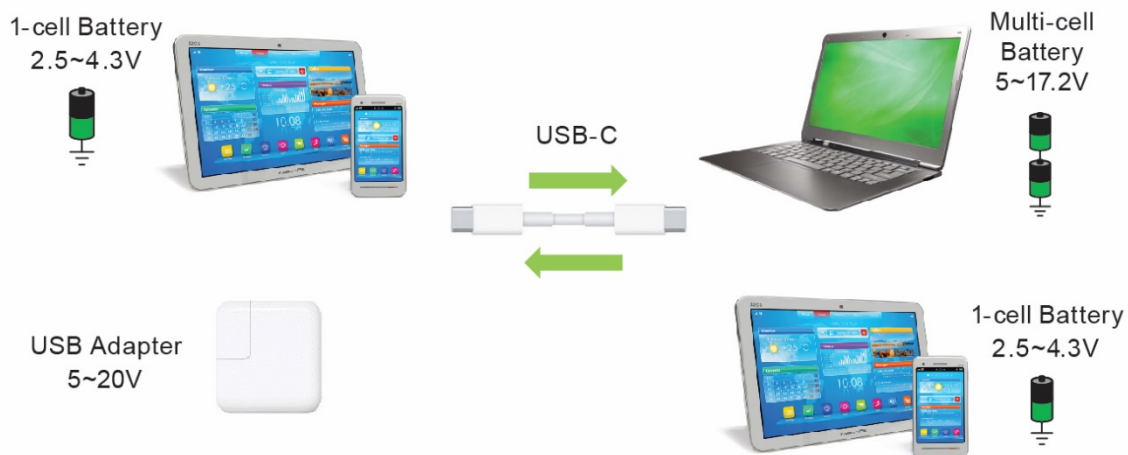
Figure 2. New power delivery architecture based on USB Type-C connector plug
