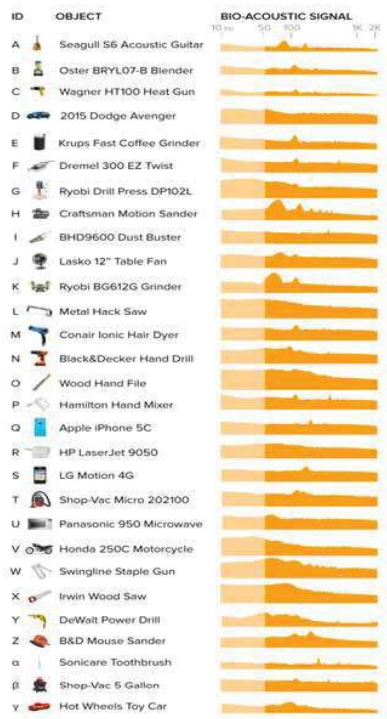
Illustration from the CMU study using vibrations captured with an overclocked smartwatch to detect what object a person is holding.
