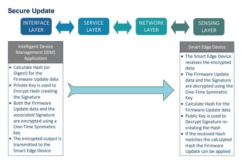
The following Security Building Blocks will typically be used on the SmartEdge<sup>™</sup> to deliver the Secure Update capability:
