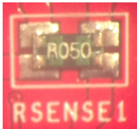
Figure 1. Picture of a Shunt (Sense) Resistor
