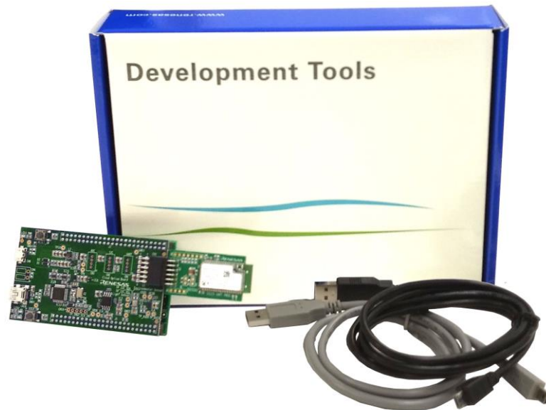
Figure 3: The Renesas RX65N Cloud Kit with cloud option board and Pmod Wi-Fi module (source Renesas Electronics Corp.)
