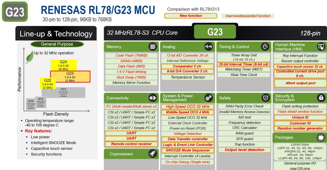
Figure 11: RL78/G23 Block Diagram
