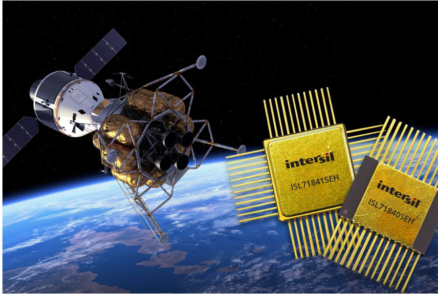
Figure 3. Rad hard ISL71840SEH 16-channel multiplexer and ISL71841SEH 32-channel multiplexer
