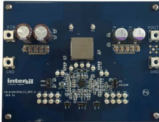
Figure 8. The ISL81601 evaluation board
