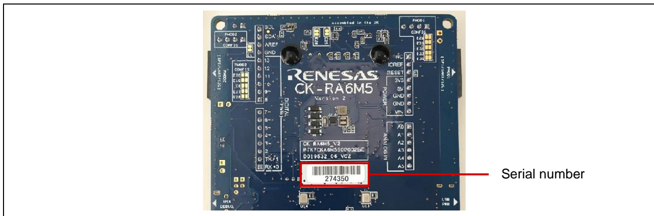
Figure 3 Location of the serial number (Bottom view of the CK-RA6M5 v2 board)
