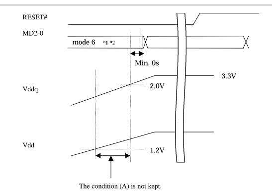
Figure 1. How to once set clock operation mode as mode 6.
